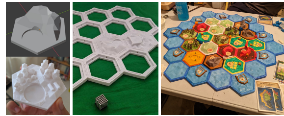
Figure 11: A hand-fabricated Settlers of Catan game. A digital model and single printed tile (left), assembling the pieces and magnets (center), playing a game (right).
